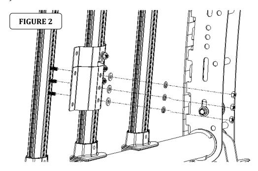
**Step-3** Place the hard case mount on the mounting brackets, align the holes and fasten with  $\frac{1}{4}$  x 1 "SEMS bolts,  $\frac{1}{4}$ " flat washers and  $\frac{1}{4}$ " hex nuts, (FIGURE 3).
